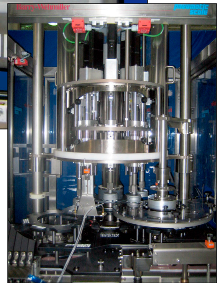
The SC Capper is available in stand-alone or monoblocked configurations.
